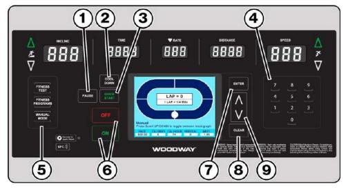
**PAUSE (1)** When the user presses the PAUSE button, the treadmill slows to a stop. The LCD will display: "treadmill paused press pause to resume". The statistics are also paused when the PAUSE button is pressed, when the user presses the PAUSE button again, the workout resumes.
