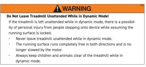
The treadmill makes it possible that the user serves as the running surface belt drive. The user drives the running surface belt manually during training. This is known as "Dynamic Mode"
