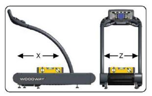
**4)** Using a 3/4" wrench make adjustments to the **Leveling Nuts (2)** at each corner until both X and Z Axis are level. Confirm leveling feet are equally weighted by carefully lifting the unit slightly at each corner.
