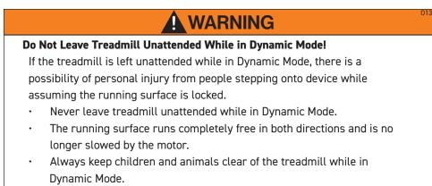
In "Dynamic Mode" the user serves as the running surface "Drive" force, by manually driving the belt surface during a workout.
