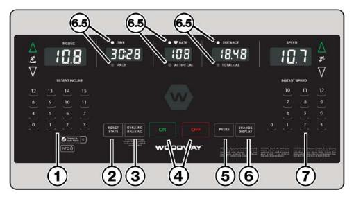
**INSTANT INCLINE (1)** Pressing any the numeric buttons 0 through 15 will set the Incline to the desired setting, without the need to press the Up/Down Incline Arrow Buttons multiple times.
