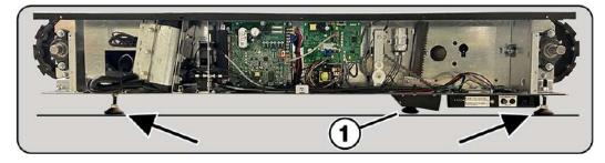
**IMPORTANT:** When making adjustments to the 4 corner points it is Very Important to keep the distance of the **Incline Foot (1)** as close to the ground as possible while leveling the overall chassis and chassis height. (incline adjustment feet should be fully retracted when doing this procedure) The distance of the incline foot should be kept at a distance of approximately the thickness of a quarter or 0.069in (1.75mm) gap from the foot to the floor.
