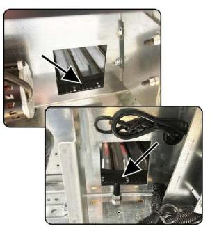
**Note:** Black Lithium Grease is recommended for lubricating the belt teeth as it is intended for more severe applications. White lithium tends to cake up and dry sooner due to additives.
