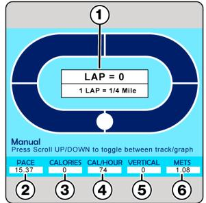
**VERTICAL (5)** Displays vertical distance calculated during workout, and based on incline levels.
