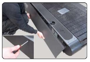
2) With both side covers removed you will have access to the Leveling Feet Lock Nuts
