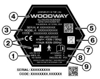
If this manual has been printed, write the Serial Number, Model Number and Model Code in the spaces below, as they will be needed when contacting the WOODWAY service department.
