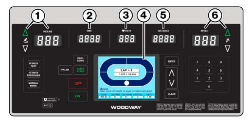
**INCLINE (1)** displays the user's current incline setting, values start at 0.0 use the Quickset Up/Down arrow buttons to increase or decrease the incline in 0.1 increments. The incline may also be adjusted using the plus/minus buttons located on the left side handrail. (Maximum incline is dependent upon the model and chosen elevation option).
