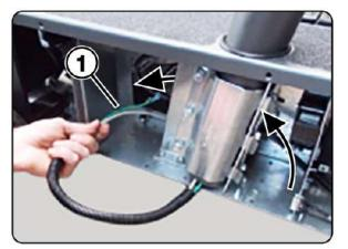
**5)** Use a 1/2 wrench to loosen the 3 nuts on each of the capture assemblies, loosen the nuts 6 to 8 revolutions each, or enough that the handrail assembly is loose enough to move.
