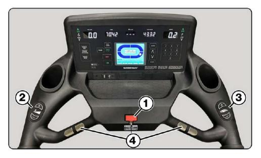
The Personal Trainer Model Main Control Console utilizes membrane style push buttons that provide users with full control over desired settings such as speed, incline, modes, and general operation.
