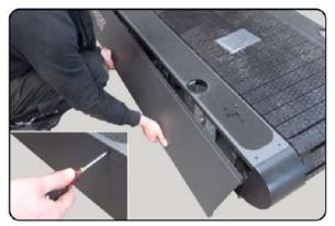
2) With the covers removed there is now access to the 3 nuts that secure the **Railing Capture Assemblies (1)** on each side of the unit.
