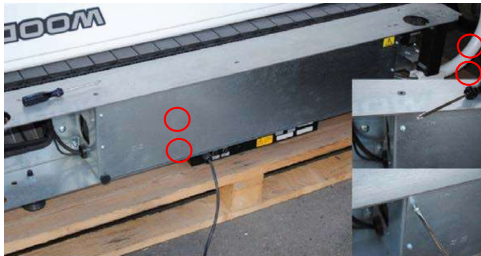
Fig. 23 Remove electronics shielding panel
