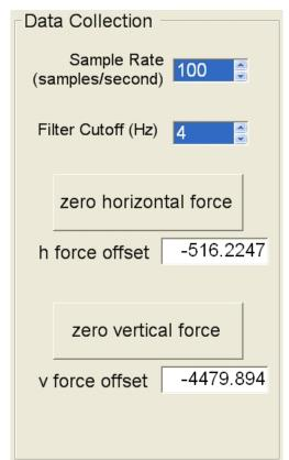
The data collection panel is used to adjust setting which affect the way measurements are made.
