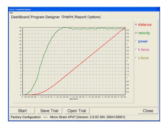
Variables that can be graphed include distance, velocity (speed), power, horizontal force and vertical force. To display a variable check the box. The color of the line is the same as the color of the variable label. Units of measurement are given on the left or right axis depending which variables are being graphed.
