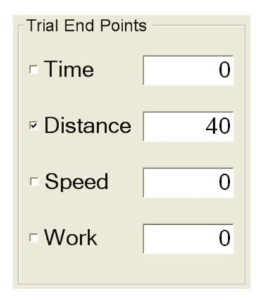
This panel is where you can set criteria to end the trial. Options include time, distance, speed attained or work done. To set an endpoint, check the box and then enter the target in the appropriate text box. Endpoints can be set on as many of the options as required with the trial stopping with the first event that occurs.
