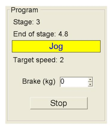
This panel displays the progress of the program if one is running. The current stage, time to the end of the current stage and the current instruction is displayed.
