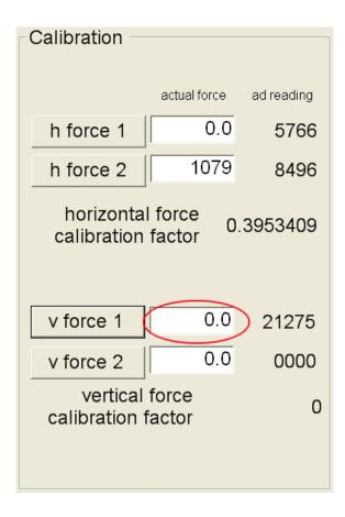
Ensure that the force entered is applied to the treadmill deck and click the button labelled "v force 1"
