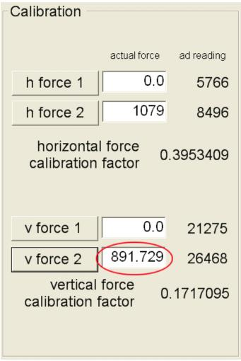
In normal use the calibration factors for both vertical and horizontal forces should be quite stable. As such calibration may only be required every few months. If the data is force scientific use and accuracy needs to be constantly verified then calibration immediately prior to the test sessions is recommended.
