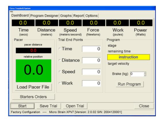
The dashboard is the main control panel for the system. Here the measurements are displayed in real time during a trial. The progress of the program if running is displayed, and the Pacer function can be used.
