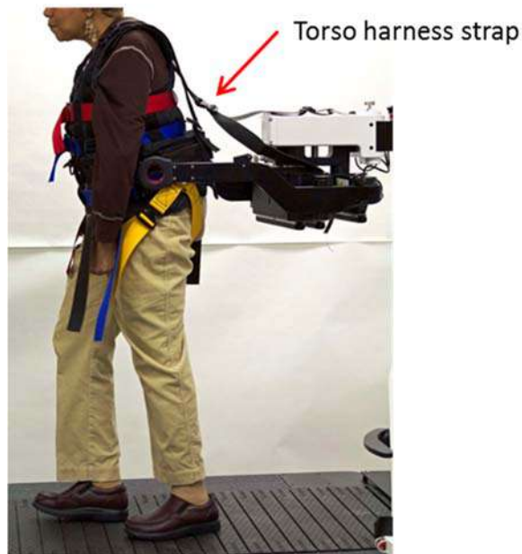
Figure 4 - Pelvic Mechanism with Torso Harness, showing torso harness and pelvic harness.
