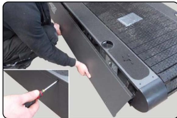
2. After removing the side covers the **Upper (1)** and **Lower Screws (2)** holding each End Cap may be removed to access the cross-shaft bearings.
