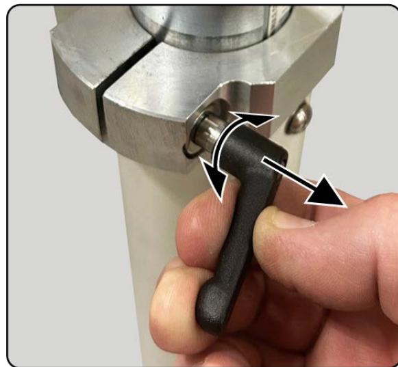
**IMPORTANT:** Whenever making adjustment with the Kip handles, ensure that when finished the Kip handle is positioned facing downwards as shown to avoid catching or snagging clothing.
