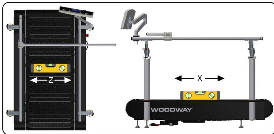
6. Using a level placed on the chassis top side plate for checking X Axis, and the level placed evenly on one of the running slats to check Z Axis.
