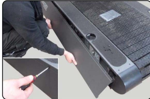
2. With both side covers removed there is access to the **Leveling Feet Lock Nuts (1)** and **Leveling Nuts (2)**. Using a 3/4" wrench loosen the **Lock Nut (1)** and turn it 5 to 6 rotations counterclockwise. This will give the needed range of movement when adjusting the height using the **Leveling Nut (2)**.
