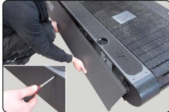
2. With the covers removed there is access to the 3 nuts that secure the **Handrail Capture Assemblies (1)** on each side of the unit.
