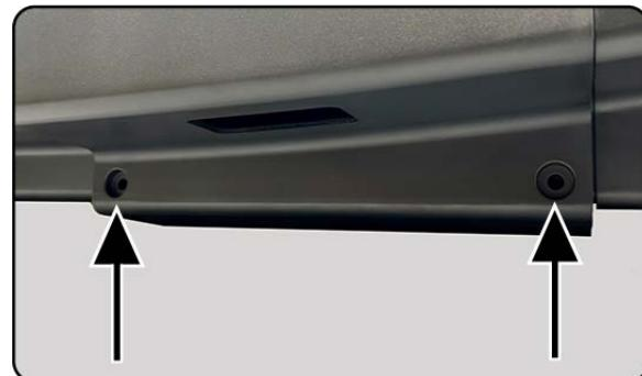
15. With the side covers installed, slide the Handrail Grommets down into position as shown.
