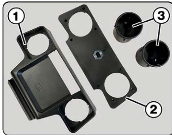
2. Install the **Control Console (1)** into the **Console Support Tray (2)** as shown. Feed the two wire harness's through the rear slot in the Support Tray. Then slide the lower portion of the Control Console into the slot at the rear of the Support Tray while rotating it into position.
