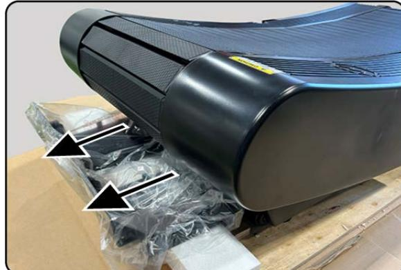
6. There are two front wheel stops nailed to the base skid support, remove them using a screwdriver or hammer to detach/pry them from the base support platform. This will aid in later unloading of the treadmill if it will be unloaded by rolling off the skid.
