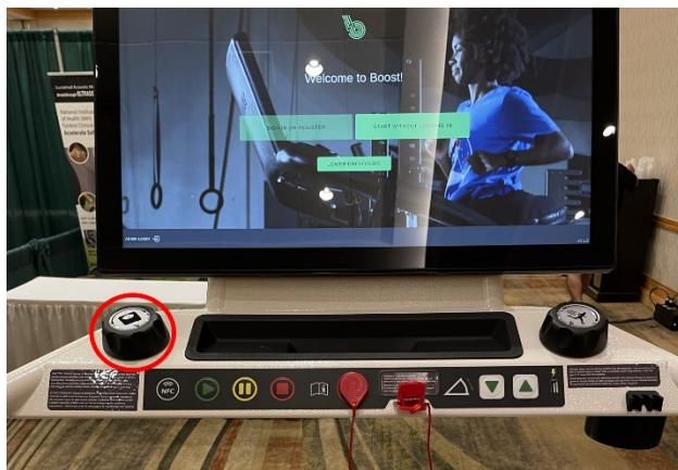
3. The red stop button finishes the deflates the enclosure, and stops the treadmill.
