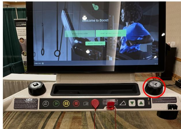
8. Reverse Mode and Free Run Mode can be accessed using the buttons in the top right of the workout screen.
