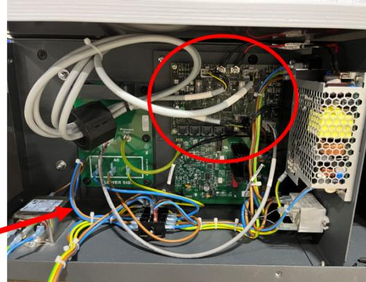
Ensure Boost 2 is powered down. To remove the fuses, remove the plastic fuse covers and pry them out of the fuse holders with a screwdriver. When replacing, ensure you have glass fuses, 4A 250V AC DC 5mm x 20mm (Bel Fuse PN 5ST 4-R). Insert the fuses back into the fuse holders by inserting one side, and then applying pressure to the other side until they click into place. Finally, replace the plastic fuse covers.
