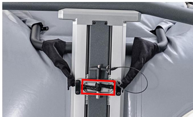
4. Test pull vertically on the release pin (without holding the release button) to ensure the release pin is securely in place before replacing the cover.
