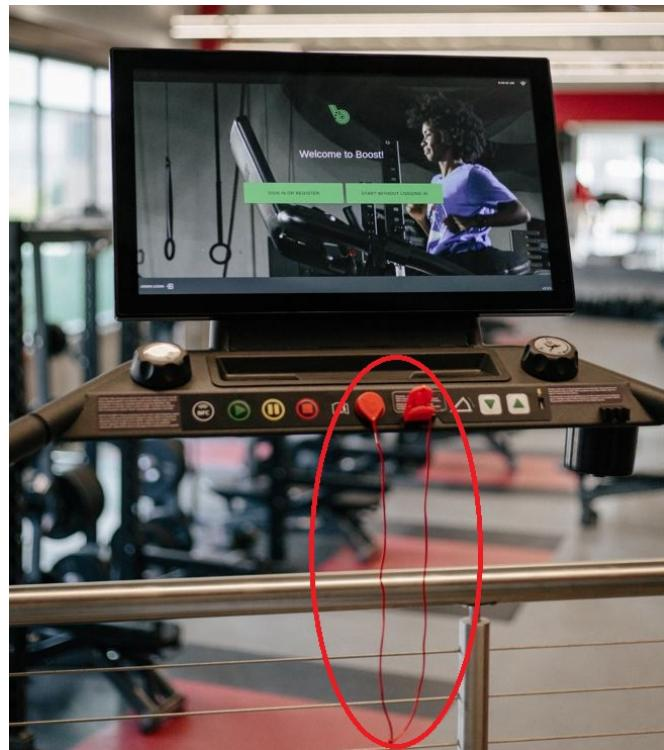
This includes shutting down the treadmill belt and incline motors, shutting down the blower, and shutting down the lift motors.
